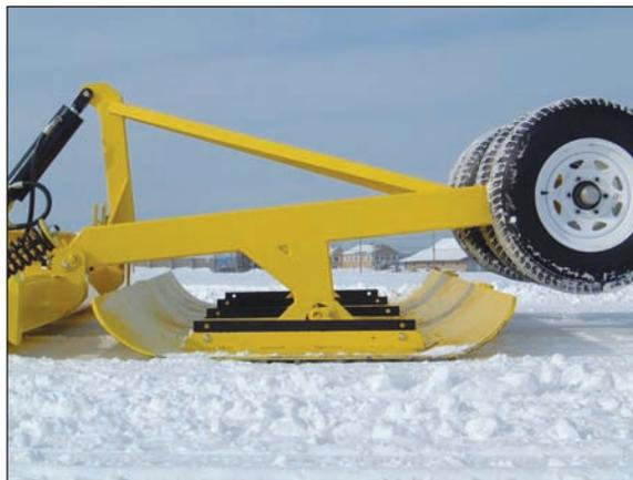
The pivot system allows the compactor to stay in a horizontal position no matter the height of the rear blades. (available on the LN and CL series)
