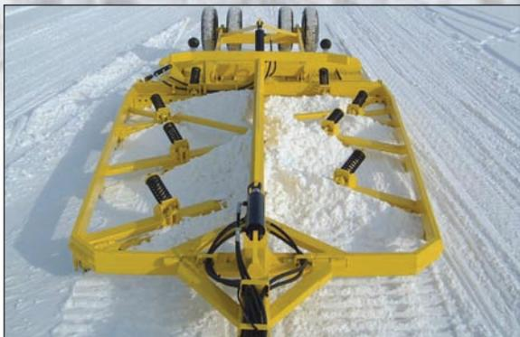
The dimensions and the total weight of the drag were verified all along the different phases of conception to allow it to be pulled by most tractor / dozers on the market.
