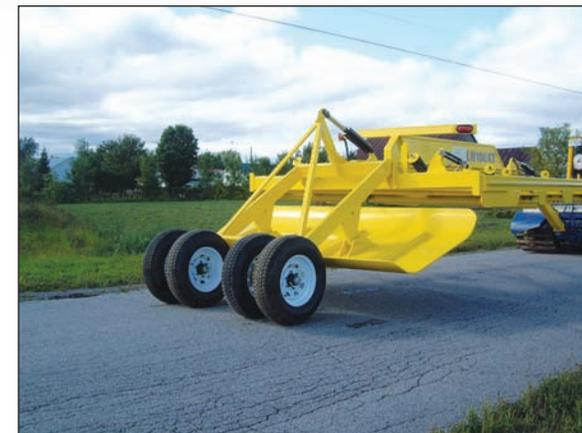
Four wheels raising system for more stability and offering more ground contact on the trail when the drag is lifted and, if a flat tire occurs, it is possible to go on. (available on the LN and CL series)
