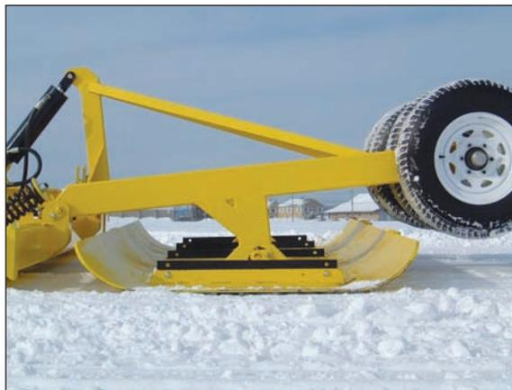
The pivot system allows the compactor to stay in a horizontal position no matter the height of the rear blades. (available on the LN and CL series)
