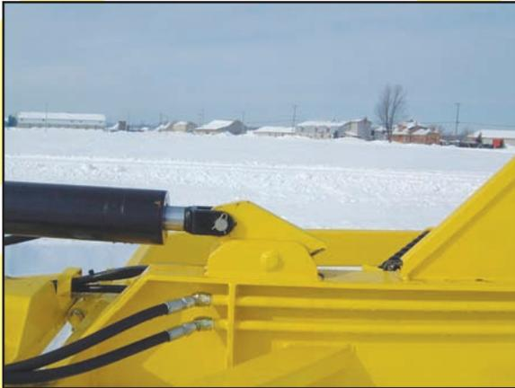
The front lever system is equipped with an anti-scalp device (available on the LN and CL series) allowing it to float or not on a hardened trail.
