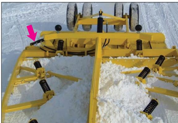
The lateral lever system (XT model), adjustable on left or right side. Allows for uniformity of trail angle when they are being widened. It also keeps the trail higher to the exterior of the curves.
