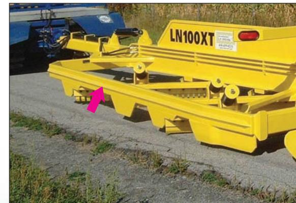
The sides are equipped with guides allowing for minimum friction to cause the least damage possible when in contact with trees. .
